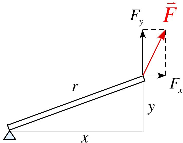
$$\vec{r} = \begin{pmatrix} x \\ y \\ 0 \end{pmatrix} \quad \vec{F} = \begin{pmatrix} F_x \\ F_y \\ 0 \end{pmatrix}$$
