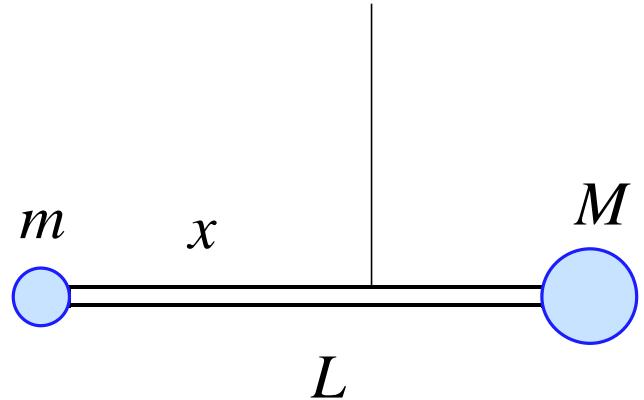
$$\vec{N}_2 = \vec{r} \times \vec{F} = \begin{pmatrix} L - x \\ 0 \\ 0 \end{pmatrix} \times \begin{pmatrix} 0 \\ -Mg \\ 0 \end{pmatrix} = \begin{pmatrix} \text{[Redacted]} \\ \text{[Redacted]} \\ \text{[Redacted]} \end{pmatrix} = \begin{pmatrix} \text{[Redacted]} \\ \text{[Redacted]} \\ \text{[Redacted]} \end{pmatrix}$$
