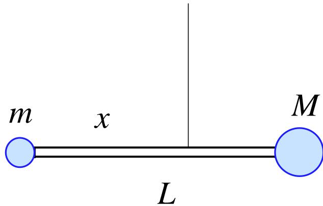
$$\vec{r} = \begin{pmatrix} -\left(x - \frac{L}{2}\right) \\ 0 \\ 0 \end{pmatrix} \quad \vec{F} = \begin{pmatrix} 0 \\ -mg \\ 0 \end{pmatrix}$$
