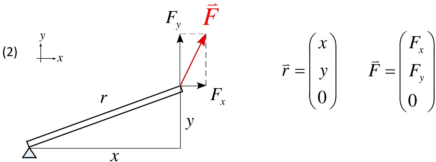
$$\vec{r} = \begin{pmatrix} x \\ y \\ 0 \end{pmatrix} \quad \vec{F} = \begin{pmatrix} F_x \\ F_y \\ 0 \end{pmatrix}$$
