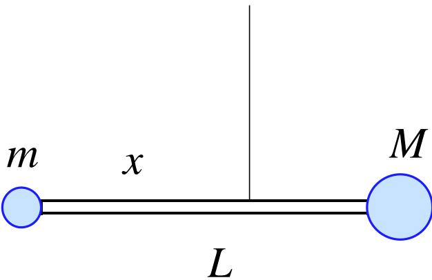
$$\vec{N}_2 = \vec{r} \times \vec{F} = \begin{pmatrix} L-x \\ 0 \\ 0 \end{pmatrix} \times \begin{pmatrix} 0 \\ -Mg \\ 0 \end{pmatrix} = \begin{pmatrix} 0 \cdot 0 - 0 \cdot (-Mg) \\ 0 \cdot 0 - (L-x) \cdot 0 \\ (L-x) \cdot (-Mg) - 0 \cdot 0 \end{pmatrix} = \begin{pmatrix} 0 \\ 0 \\ -(L-x)Mg \end{pmatrix}$$
