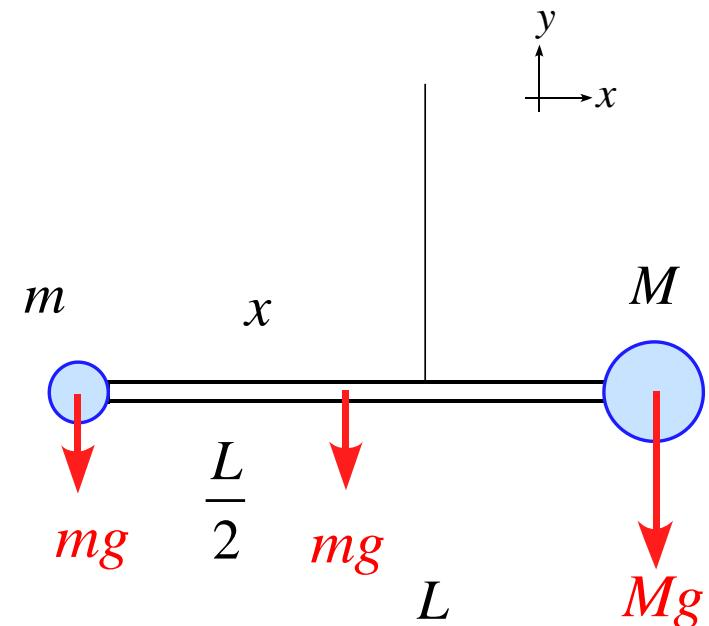
$$\vec{N}_1 = \vec{r} \times \vec{F} = \begin{pmatrix} -x \\ 0 \\ 0 \end{pmatrix} \times \begin{pmatrix} 0 \\ -mg \\ 0 \end{pmatrix} = \begin{pmatrix} 0 \cdot 0 - 0 \cdot (-mg) \\ 0 \cdot 0 - (-x) \cdot 0 \\ -x \cdot (-mg) - 0 \cdot 0 \end{pmatrix} = \begin{pmatrix} 0 \\ 0 \\ xmg \end{pmatrix}$$
