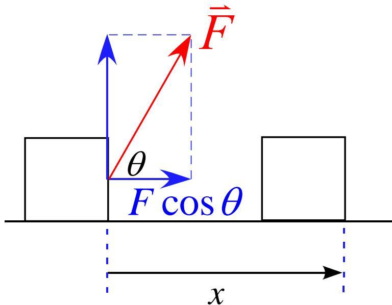
$$\begin{aligned} W &= F \cos \theta \times x \\ &= Fx \cos \theta \end{aligned}$$
