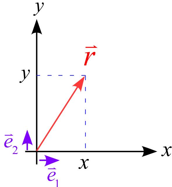
$$\vec{r} = (x, y) \quad \vec{r} = \begin{pmatrix} x \\ y \end{pmatrix}$$
