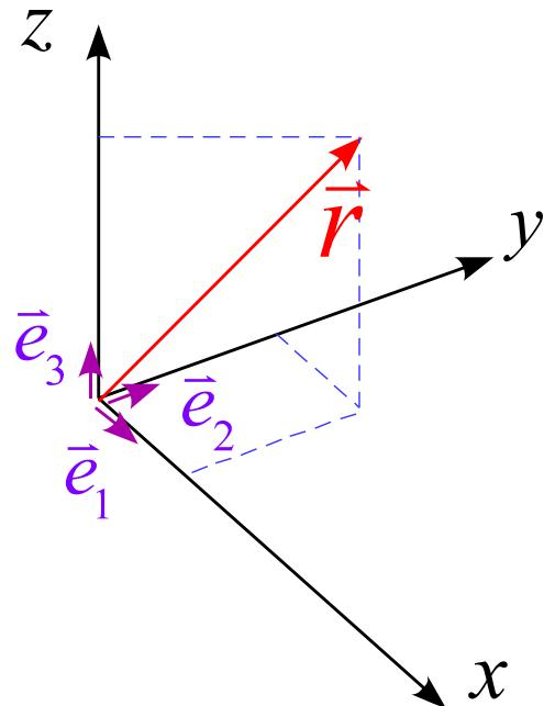
$$\vec{e}_1 = \begin{pmatrix} 1 \\ 0 \\ 0 \end{pmatrix} \quad \vec{e}_2 = \begin{pmatrix} 0 \\ 1 \\ 0 \end{pmatrix} \quad \vec{e}_3 = \begin{pmatrix} 0 \\ 0 \\ 1 \end{pmatrix}$$
